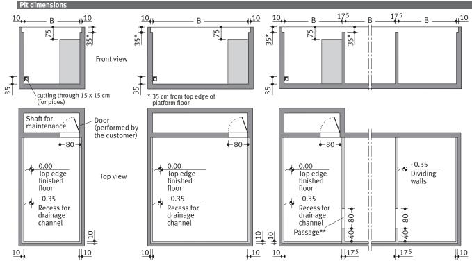
Access to adjacent systems must be level with the maintenance shaft access to the pit
