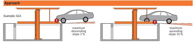
The illustrated maximum approach angles must not be exceeded. Incorrect approach angles will cause serious maneouvring & positioning problems on the parking system for which the local agency of Klaus accepts no responsibility.
